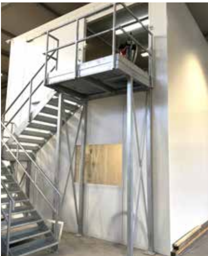
Soundproof enclosure for a concrete block machine
