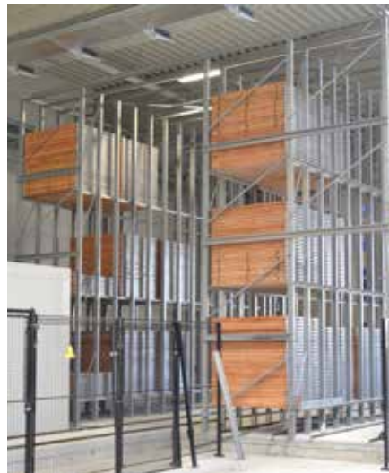
Board buffer rack for storing production boards
